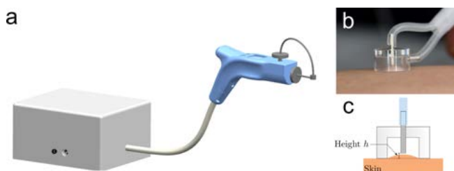
Figure 1: (a) The new NIMBLE consists of a measurement station (white), a handheld (blue) and a disposable (grey). (b) For a measurement the probe is placed on the skin and a vacuum is created, (c) the vacuum elevates the skin until a predefined height h is reached. The pressure required is a precise indicator of skin stiffness.
